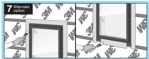
An alternative method is to use 3M<sup>™</sup> Adhesive Sealant 740UV to seal over the flange on either side and across the top, extending a minimum of 2" onto the wall membrane. Apply the bottom membrane leaving approximately 2" open on either side to allow drainage should moisture get behind the flange.
